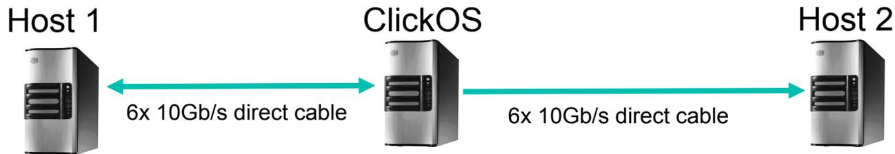
Intel Xeon E1650 6-core 3.2GHz, 16GB RAM, dual-port Intel x520 10Gb/s NIC.
